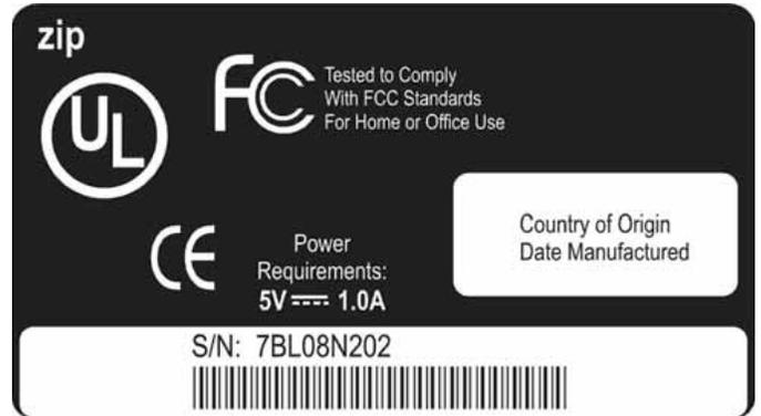
Often, the letters UL are on the nameplate. UL stands for Underwriters Laboratories, Inc., which conducts tests on thousands of machines and appliances. The UL mark means that samples of the machines and appliances have been tested to make sure they are safe.
