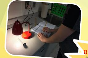
We measured the temperature of the bulb after each minute for 10 minutes and recorded our results on a chart. LED light bulbs produced the least thermal energy in 10 minutes and wasted the least energy.
