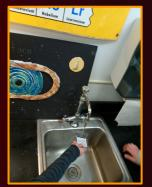
Using flowmeter bags to determine the water flow out of the school sinks
